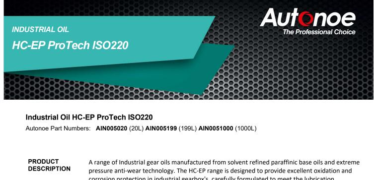
corrosion protection in industrial gearbox's, carefully formulated to meet the lubrication requirements of a wide range of enclosed gear tooth configurations such as spur, bevel, helical, double helical, worm, spiral bevel, and hypoid.
