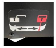
Scale lock indicator showing scale is unlocked.
